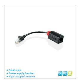
The PoE Finder detects the existence of PoE power supply and the proper functioning of PoE, which simplifies the detection and recognition PoE network. It differentiates between mid-span(4/5/7/8) and end-span(1/2/3/6) PoE power supply and supports IEEE802.3af/at standard PoE and passive PoE. It provides male and female connectors, able to detect PoE port or cable directly. The LEDs lit up or flash once plugged in the powered network. The easy installation makes it convenient for construction.
